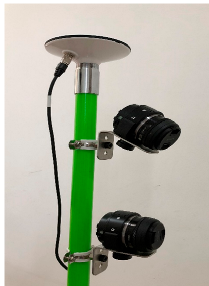
Figure 4. Two CCD lens placement details.
